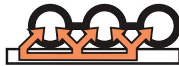
The 'heat trap' design enables stored energy to be radiated directly from the roof to the water channels.
